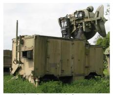
**BMPG's Radar Type 86 before recovery** The above photo shows the condition of the T86 before recovery. Note: The two covers on the rear of the Aerial Assembly have now been replaced. The missing on-launch reference aerials, on the corners of the cabin, have also been replaced.
