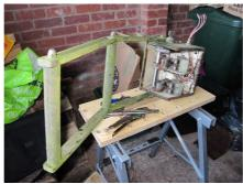
Roof Ladder in the 'Workshop' In the photograph above the 'new' Castell Key is protruding from the top of the roof switch box.
